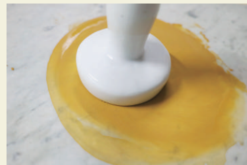
3. Paraloid™ B 72溶液と顔料を練り合わせる Mix Paraloid mixture and pigment together and stir well
